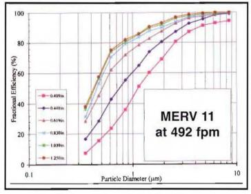
Particle Size Removal Efficiency Conducted by LMS Technologies. Filter Size: 24 x 24 x 24 - 6 pocket
